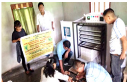
Installation of 1000 eggs capacity Poultry Hatchery unit cum trial at CHC, Purangang village.
